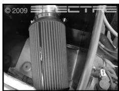
Step 13 Install the filter onto the intake tube and secure with the supplied clamp.
